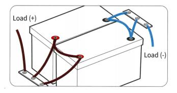
After parallel connection, the capacity of the battery system will be doubled according to the number of batteries you connect. E.g. If tw 12V100Ah batteries are connected in parallel, the battery system will be 12(12.8V)200Ah
