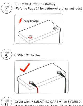
Please do not cover the post bolts with insulating caps when using the battery.
