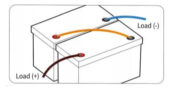
After series connection, the voltage of the battery system will be doubled according to the number of batteries you connect. E.g. If two 12.8V100Ah batteries are connected in series, the battery system will be 24V (25.6V)100Ah
