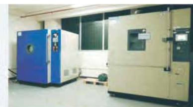
Low Pressure Test Chamber (L) Constant Temperature and Humidity Test Chamber (R)
